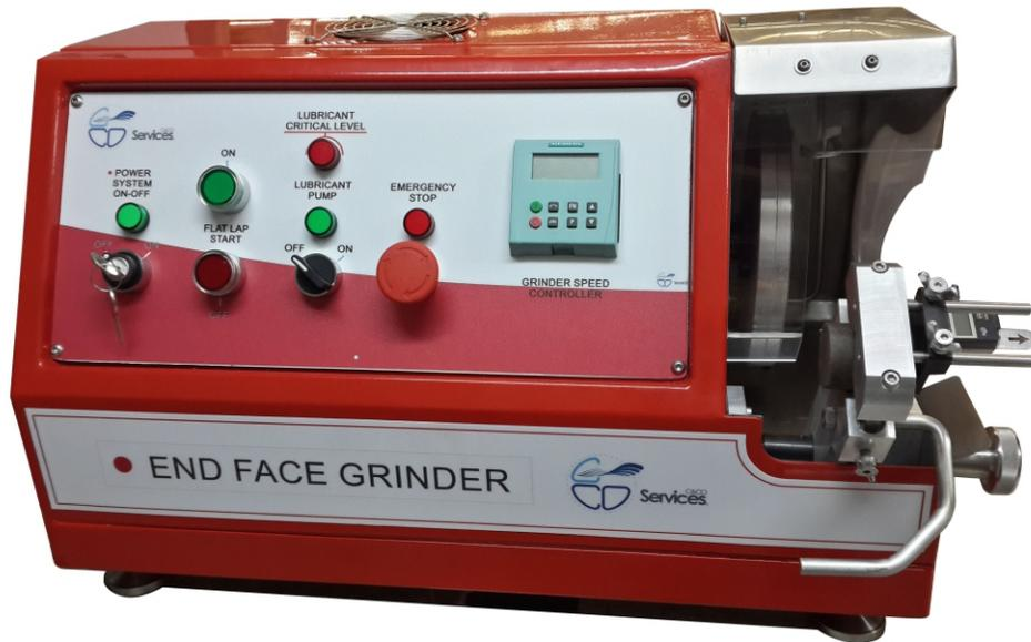
The End Face Grinder (PCT-100) allows polishing the surfaces of each core plug sample with an accuracy of 0.01 mm to rectify those plugs after Trimming process with imperfections. This unit allows to totally parallel faces of the caps with an accuracy of about 0.01 mm, generating perfect cylinders for determining the volume of each plug with high precision.
