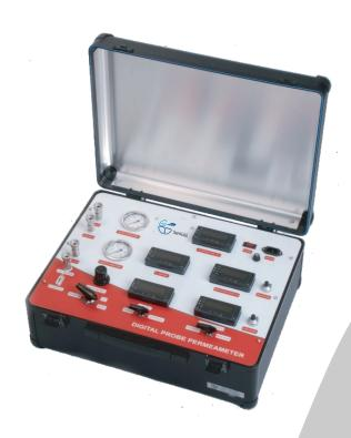
The digital probe permeameter is a portable and versatile laboratory instrument to be used in fields and labs. The main advantage of the permeameter is its proven ability to realize specific, quick and non-destructive measurements of gas permeability from a great variety of core surfaces (slabbed and whole cores, plugs, fragments, etc.) other advantages are:
