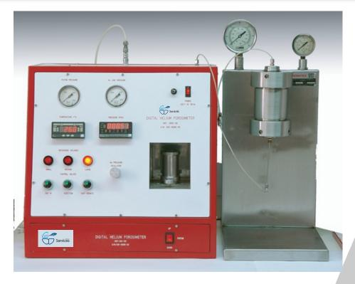
Analytical degree laboratory equipment, used to measure the Grain Volume and Pore Volume in rock samples. With the data measured by the equipment, plus the weight and bulk volume of the sample, the porosity and grain density of rocks is calculated. Its measurement principle is based on Boyle's Law for gases at constant temperature.
