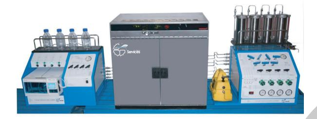
With C&CO SERVICES S.A.S FLOW THROUGH CORE CLEANER you could implement a fast and efficient cleaning system for cores and rock samples, based on controlled sequential solvent displacement under established pressures and temperatures. The extraction of hydrocarbons and salts from reservoirs rocks is achieved by injecting one or more solvents into the core sample under pressure and moderate temperature.
