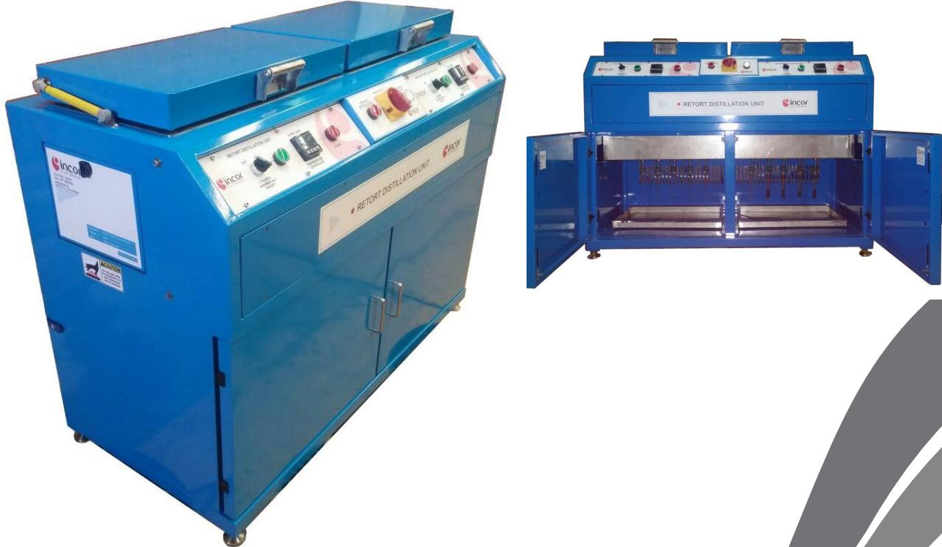
This equipment is comprised of a two-chamber oven allow to handle up to 20 samples of 100 grams or 20 samples of 10 grams (for determination of fluid saturations of wall samples). The retort has an electronic controller that lets you program and control the temperature, in addition, it has a water condenser. The equipment can take direct readings of the volumes of water and oil containing samples. Includes a set of graduated test tubes (2cc and 10cc).
