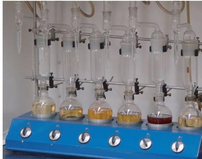
**Dean Stark:** Is an analytical laboratory Equipment, used to measure the fluid saturation of rock samples. Through solvents, the water and oil that saturate the sample are extracted and distilled; the product of the distillation is condensed over a calibrated trap which by decantation separates water from the solvent and allows quantification.
