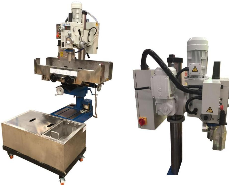
Automatic drill to take rock samples of up to Ø 2 ½" and 5" of length.
